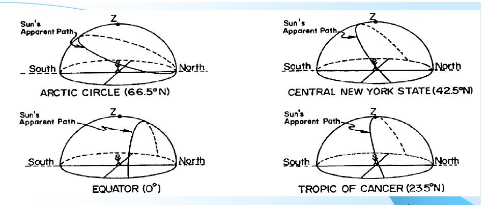
Sun's apparent path for four different observers on June 21<sup>st</sup>. Notice how the path and position of the noontime sun change for each location.
